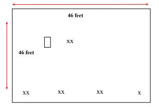
Key - xx - Double Plug Socket x - Single Plug Socket
